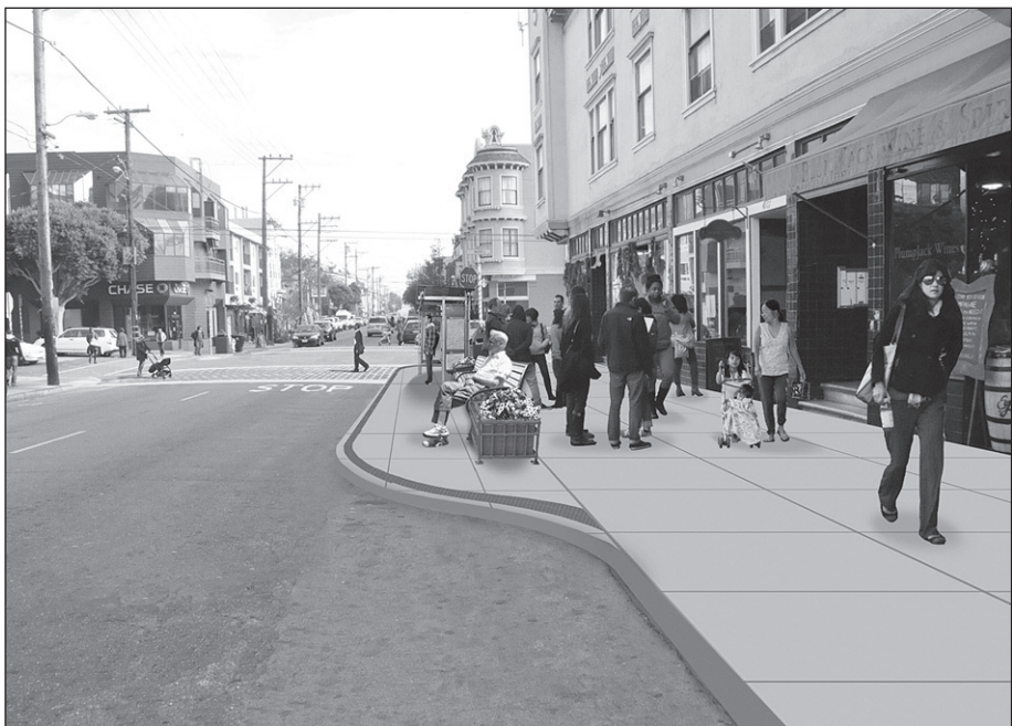
This artistic rendering of a proposed bulbout at 24th and Noe streets shows how an additional seven feet of sidewalk shortens the length of the crosswalk and enables buses to load and unload passengers without leaving the traffic lane. Rendering courtesy Jason Su, DPW
